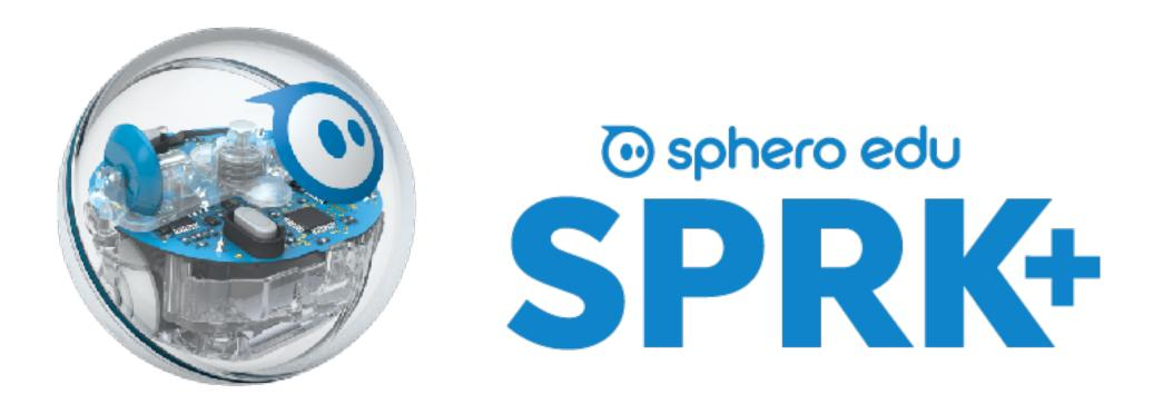
Shell: Clear, durable, waterproof, scratch-resistant, sealed Charging: simple, inductive charging Learn Time: 1 hour Sensors: Gyroscope, accelerometer, and motor encoders Connection: Bluetooth LE (30m) Compatibility: Sphero Edu app, Sphero app Size: about as big as a baseball Speed: 4.5 mph Accessories: maze tape, protractor, sticker sheet
